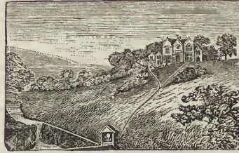
View of Ram worked by water from a spring, and supplying the house and garden on the hill.
